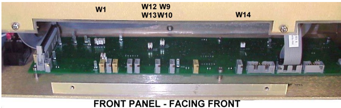
Figure 5-1: XDS Configuration Jumper Locations
