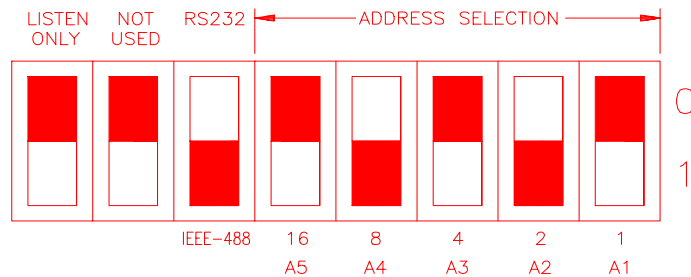
Figure 9-3: GPIB Address Selection Switch
